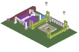
**5** Check that the socket on the target system is still open.
