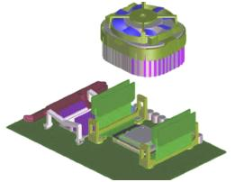
15 Install the clip assembly to hold the heatsink in place.
