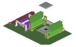
$11\,$  Align the processor over the socket on the interposer.
