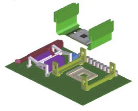
Note how the socket on the interposer is rotated 180° relative to the socket on the target system. This is done so that the interposer will not interfere with the target socket's actuation mechanism.
