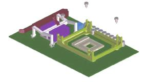
**4** Install the Agilent retention modules.
