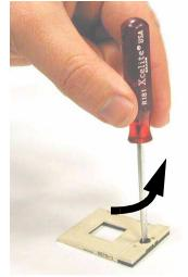
6 Remove the pin protector from the interposer.
