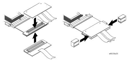
17 Connect the analysis probe to the logic analyzer.
