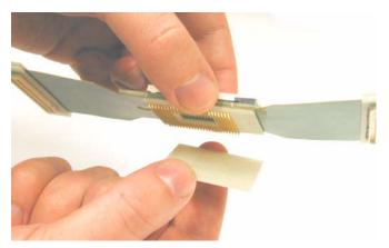
7 Align the interposer over the socket on the target system.
